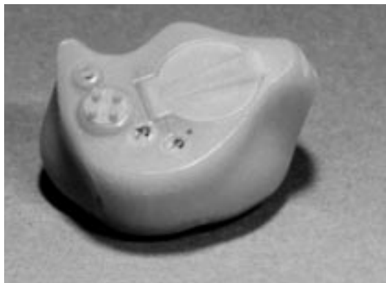
Figure 6 This shows an in-the-ear hearing aid.
