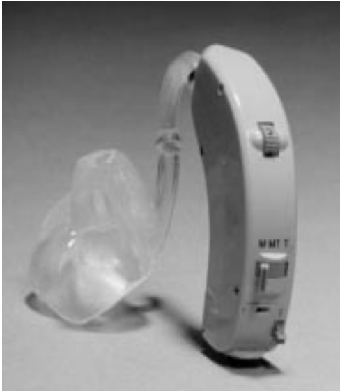
Figure 7 This show a BTE (behind-the-ear) hearing aid. The earmold is shown on the left of the illustration.
