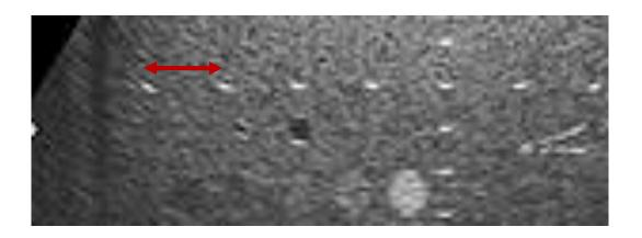
Vertical Distance - Measure the distance, center to center, of two pins that are 4-10 cm. apart vertically.
