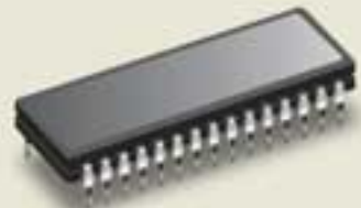
BIOS The BIOS above is a small chip found on every motherboard. It is much smaller than the up-close version we depict on these two pages.
