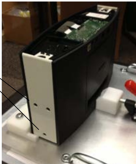
Figure 27. Reman SoundTouch® 20 Top Cap and Grille Alignment Fixture.
