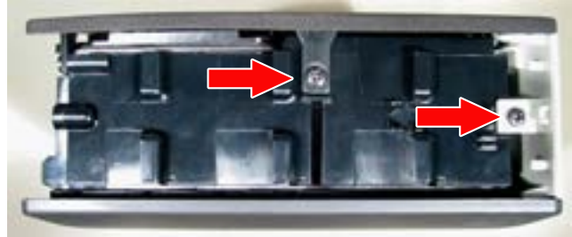
Figure 8. Grille and Top Cover Removal, Side Screws.
