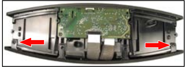
Figure 7. Grille and Top Cover Removal, Bottom Screws
