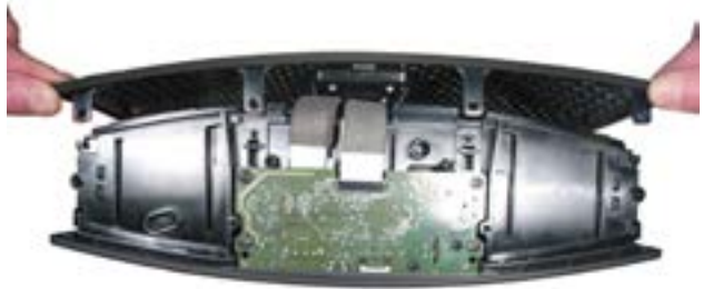
Figure 9. Grille and Top Cover Removal
