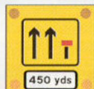
Signs used on the back of slow-moving or stationary vehicles warning of a lane closed ahead by a works vehicle. There are no cones on the road.
