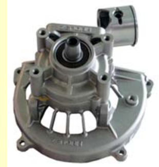
Reduced excess material of crankcase to reduce weight leaving support rib
