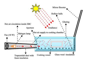
Fig. 1. Schematic diagram of the modified SBC.
