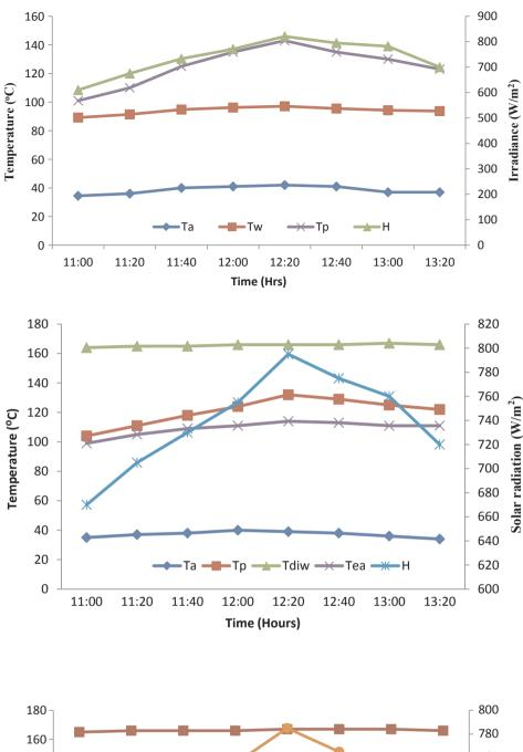
Fig. 5. Sensible testing of new SBC on configuration 2.
