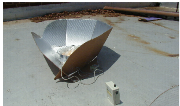
Fig. 2 A panel solar cooking kit showing a sealed pan, a data logger in the shade and a pyrometer in the foreground
