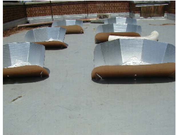
Fig. 1 A photograph showing the arrangement of the panel solar cookers during the study
