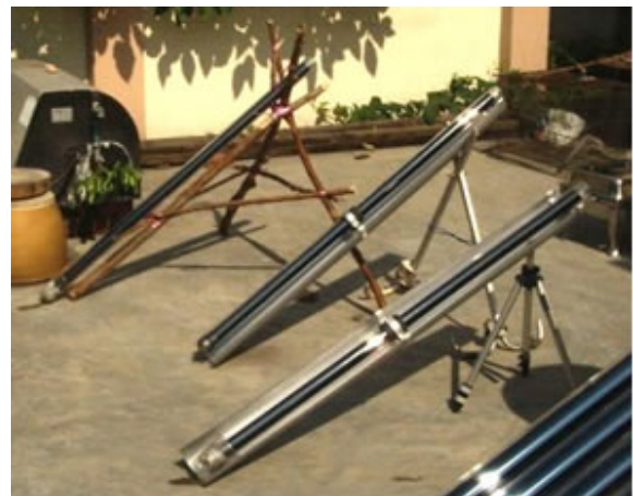
Figure 7: Improved with Local Material Possibilities: Lashed Jungle Wood Tripod Stand, Re-used discarded baby pram metal, camera tripod stand, plastic cups etc
