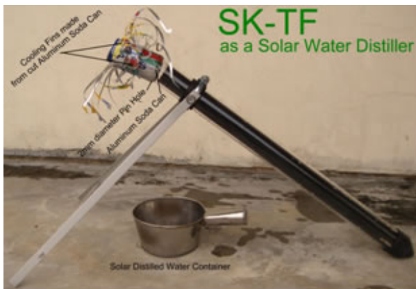
Figure 11: The SK-TF as a Solar Water Distiller
