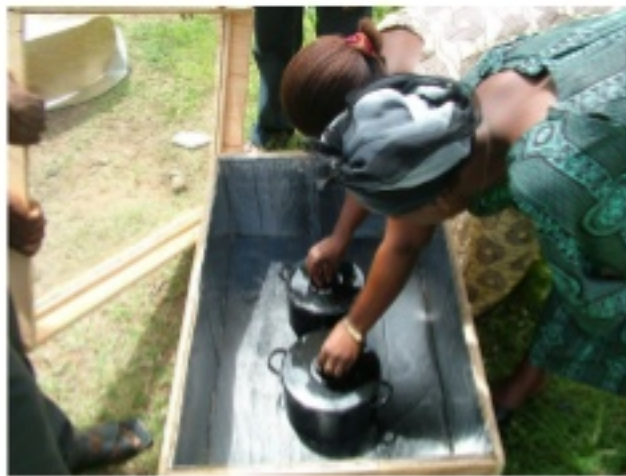
Figure 2: Box Solar Cooker with Glass Lid, Ago-Are, Nigeria (with Rukayat Adewumi, front, and Grace, back)
