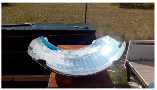
The secondary reflector made of aluminum sheets.
