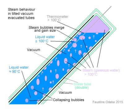
Please consider this particular behaviour, especially when you apply vacuum tubes with a small diameter, to avoid scaldings.
