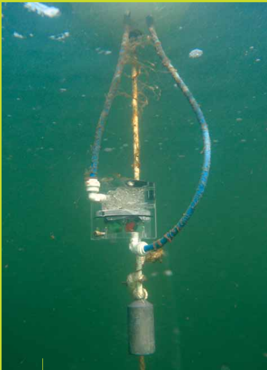
Figure 4. A microbial fuel cell operating in seawater (Developed by the Air Force Research Laboratory and the US Naval Research Lab).
