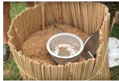
Fig. 9. Photo of ISEC built in Uganda. A reed mat was used as the outer structure. The heater rests inside a larger pot as shown. A smaller pot holding the food rests on top of the heater and a ceramic tile under the larger pot insulates the rice hulls from the hot spot beneath the heater.
