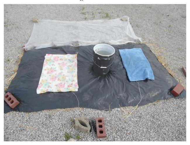
This photo shows the test set up for killing insect eggs. Two temperature loggers are under the clothing, one on the left and one on the right. The stack on the left is 3 pillowcases on top of each other, and the stack on the right is a thick towel folded into thirds. A bucket of water is used to support the top clear plastic layer, and because heating wash water is a common need for many people.
