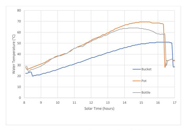
This shows the temperature vs. time curves for water containers of various sizes. Note that the pot achieved  $70^{\circ}$  C, more than halfway to the boiling point.
