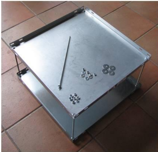
Fig. F2 Workplace for Ben-stove on a rack with two platforms held by four threaded bolts with alternative pieces for fastening the platforms on the bolts: nuts, self-locking nuts, washers and the (preferred) serrated nuts. Tubes passed by the bolts are also possible.
