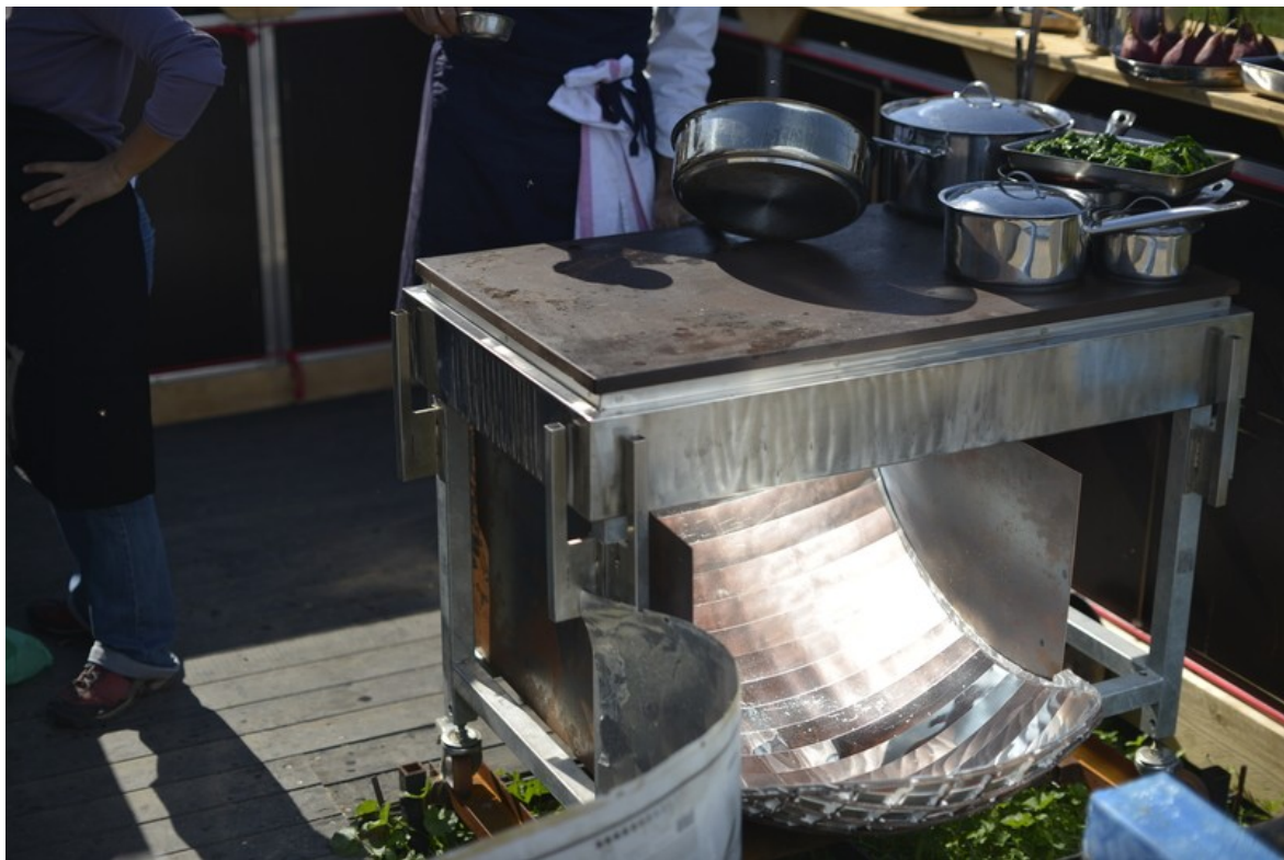
The secondary reflector made of aluminum sheets and fitted into the stove.
