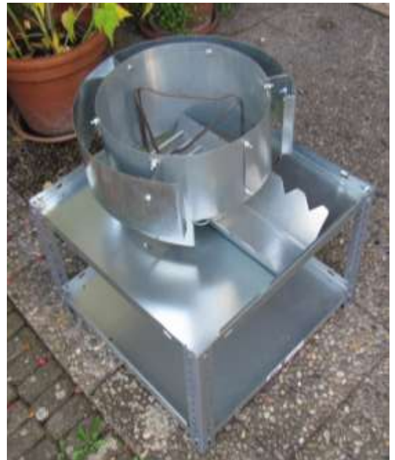
Fig. 2. Bolted shelf for firewood stove Ben 2 or Ben 3. Dimensions of the shelf: 50 cm x 50 cm, height 33 cm. The shelf is produced from prefabricated components of Vario System, Schulte
