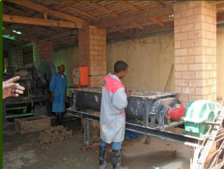
The kneading machine in operation
