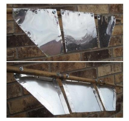
Metal reflector (e.g., anodized aluminum) bent-over perimeter edges adds stiffness to the facets and avoids sharp metal edges and has 3-ply metal layers at the bolt connections.
