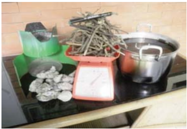
Fig. 3: left: Small pieces of firewood, middle: Paper briquette (pb), right: 100 gram pb and 210 gram small wood are used in the green stove for boiling 5 litres of water.
