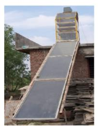
Photograph 4: Low cost solar dryer for agro processing.
