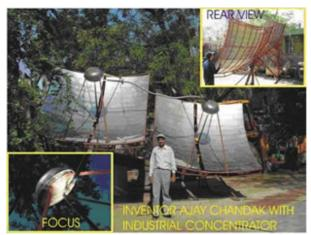
Photograph 2: 'Industrial Solar Concentrator' for hot air up to 200<sup>o</sup>C
