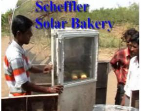
Photograph 3: Oven used for bakery using Scheffler Concentrator.
