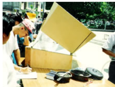
Fig. 13 Multi reflector Inti 2000. Rodrigo Carpio 1994, second place in the Third Annual Solar Cooker Contest. California. Home Power Magazine. ISSUE No. 43
