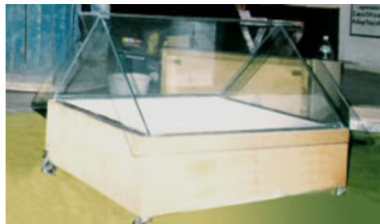
Fig. 6 Greenhouse effect conventional solar dehydrator.
