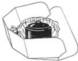
Fig. 9 Solar Cookit. Model SCI 1997 and "Sun Toy" SCI. (However, the slope of the reflector's central segment (more than 90 degrees) does not favor reflection in low solar altitude positions).
