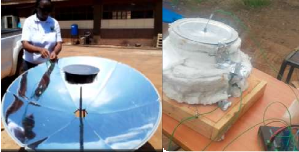
Figure 2: Thermal energy storage on a solar cooker during charging (left) and discharge cycles (right).
