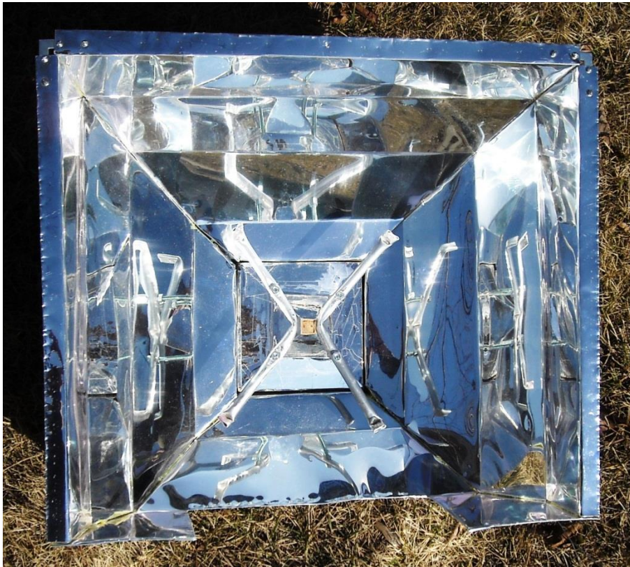
Anodized aluminum reflector mock-up full-size model with 3lb SCI roaster
