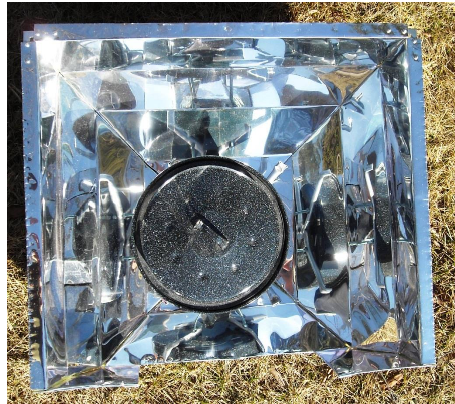
Anodized aluminum reflector mock-up full-size model with 3lb SCI roaster
