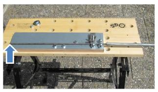
Fix the round steel (617 mm length, 6 mm diameter) at the bending device with the clamping piece and the wing nut. Align left end of the rod with the left side of the plate.
