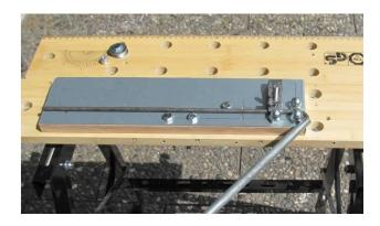
First bend with the help of the tube as lever
