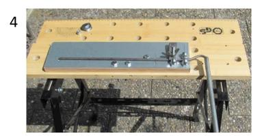
Second bend with the help of the tube as lever
