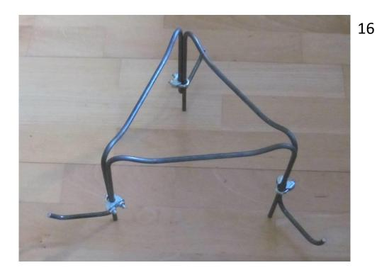
Rope clamps may provide a alternative for connection of the tripod legs if welding equipment is not available.
