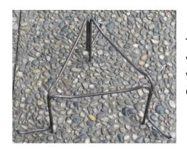
Three tripod legs are welded together;
