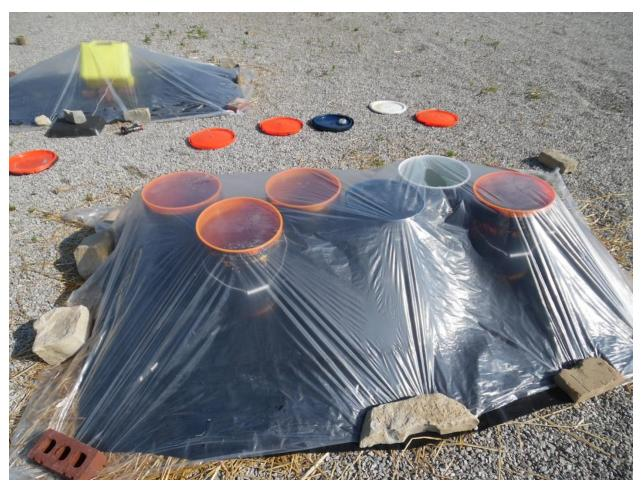
The system with the clear top layer added. This unit has 6 buckets of water. Typically, 4-6 rocks are used on each long edge, and 3 or so are used on the short edges. This provides a seal around the edges that is good enough to hold in the heat, but loose enough that there is some air circulation to carry away moisture. The plastic is snug on the top of the buckets to prevent much evaporation.
