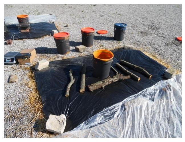
This photo shows a single bucket of water to be heated and 6 pieces of wood to be dried. Put the objects to be heated on top of the black plastic.
