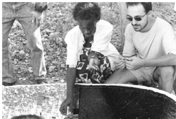
Small glass mirror pieces are applied to the cooker shell in mosaic form.
