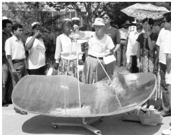
A Chinese-style cooker shell, molded from clay by artisans in Nepal. (Photo courtesy of Hannu Virtanen.)
