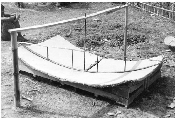
A Chinese-style cooker shell, molded from clay by artisans in Nepal. (Photo courtesy of Hannu Virtanen.)
