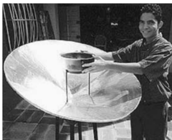
Herbert Aguilar demonstrates a small parabolic cooker.
