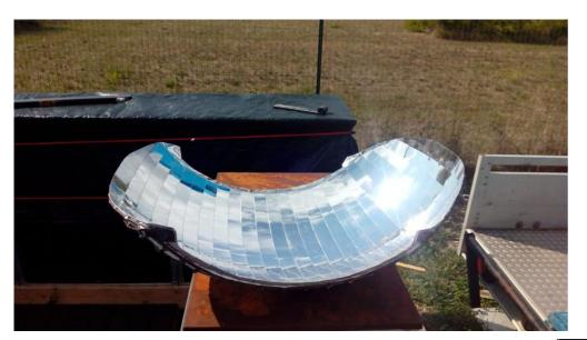
The secondary piror is made of aluminium foil.
