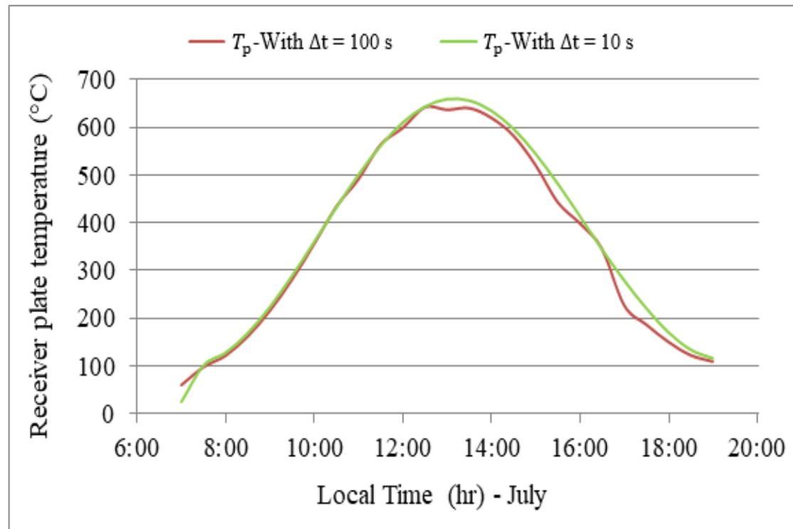
Time variation of the receiver plate temperature at different time steps
