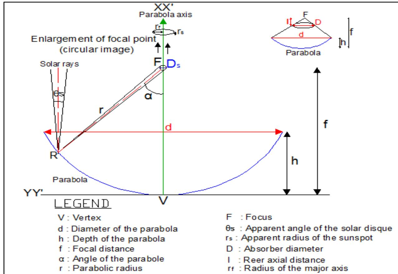
Geometric elements of the parabola
