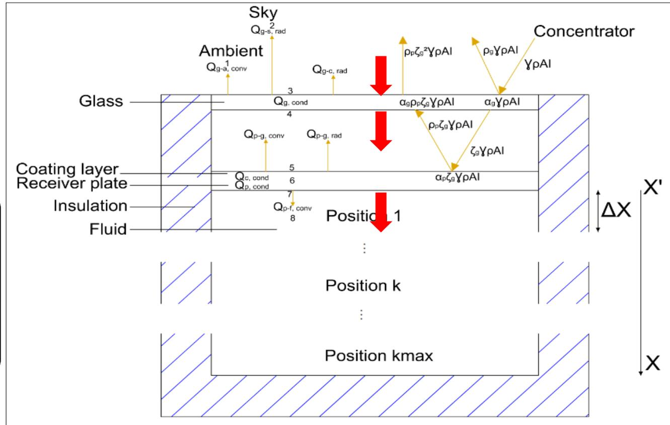
Cross section of the receiver with heat transfer processes
