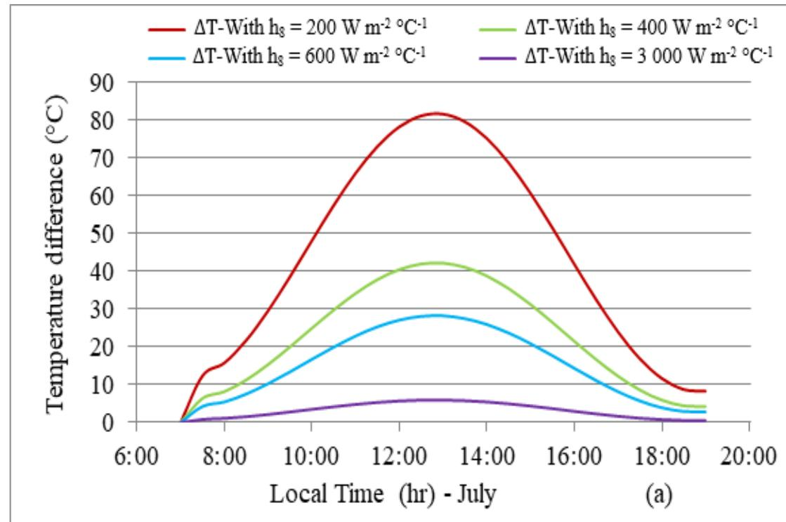
Time variation of the temperature difference between the plate and the fluid when increasing the heat transfer coefficient
