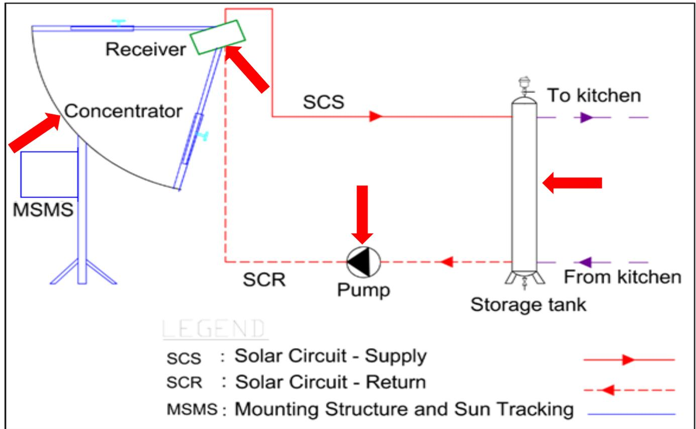
Schematics of a solar cooking system with heat storage
