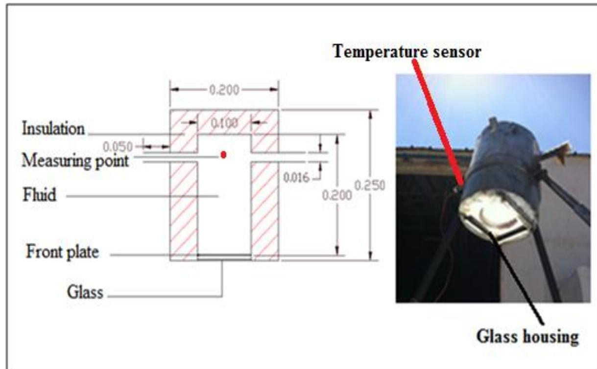
Longitudinal section and photograph of the absorber
