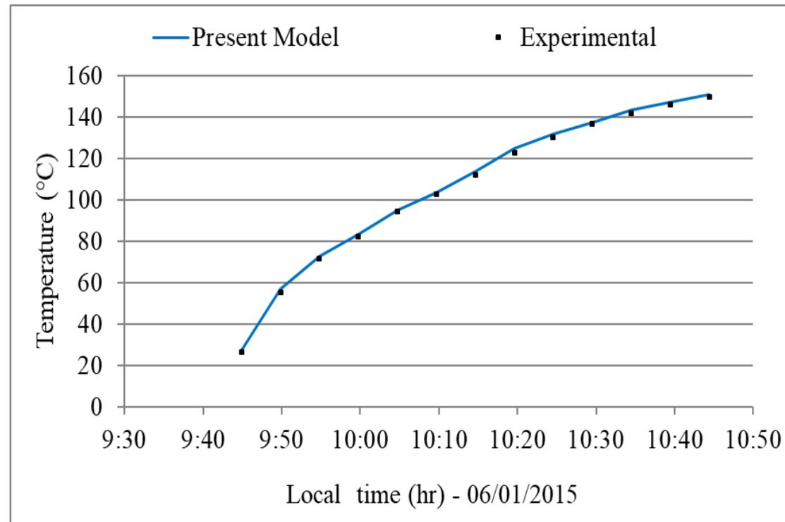
Measured and predicted fluid temperature in the receiver in closed circuit of the second experimental device
