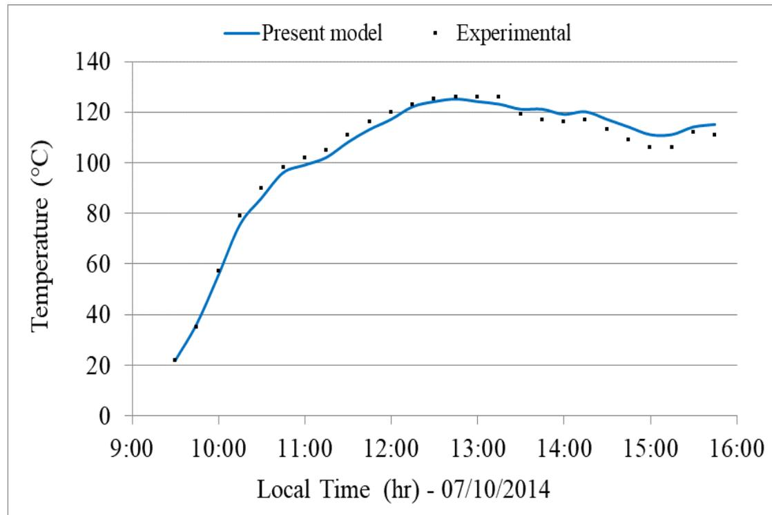
Measured and predicted fluid temperature in the receiver in closed circuit of the first experimental device
