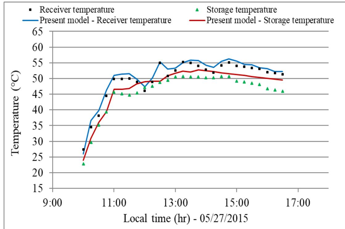
Measured and predicted fluid temperature in the receiver and in the storage tank in open circuit of the second experimental device
