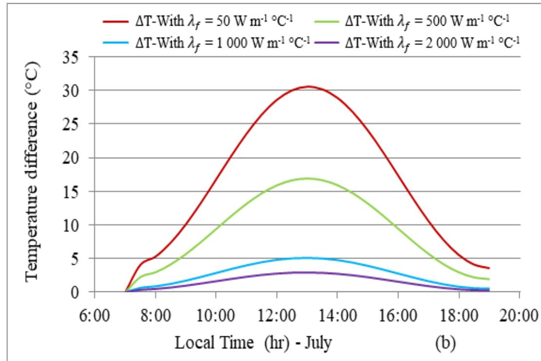
Time variation of the temperature difference between the plate and the fluid when increasing the fluid thermal conductivity
