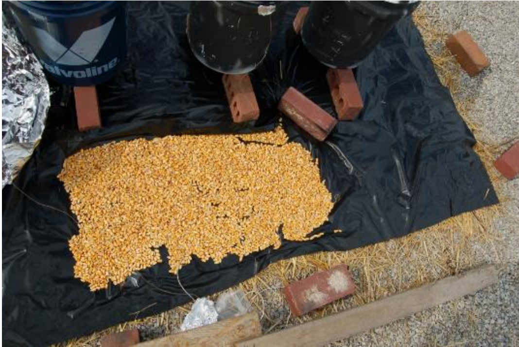
Figure 18: This shows how 3 kg of corn can be dried while performing other tasks simultaneously. This photo shows an early design when bricks were still being used under the water buckets. Later designs omitted these bricks and improved the performance.
