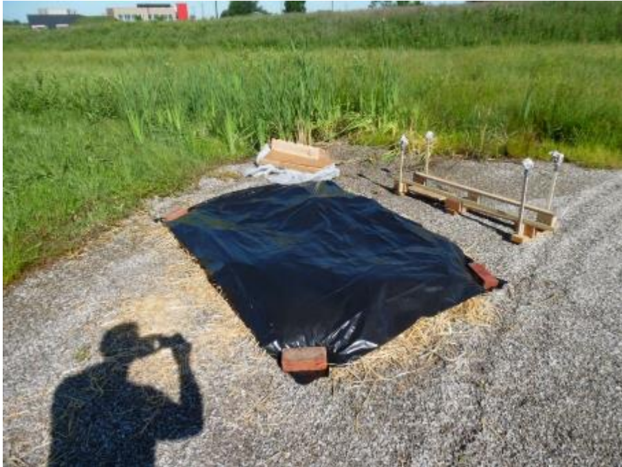
Figure 3: Cover the organic material with a layer of black plastic or similar material. In the background is a wooden structure that was used in early tests, but is not part of the final design.
