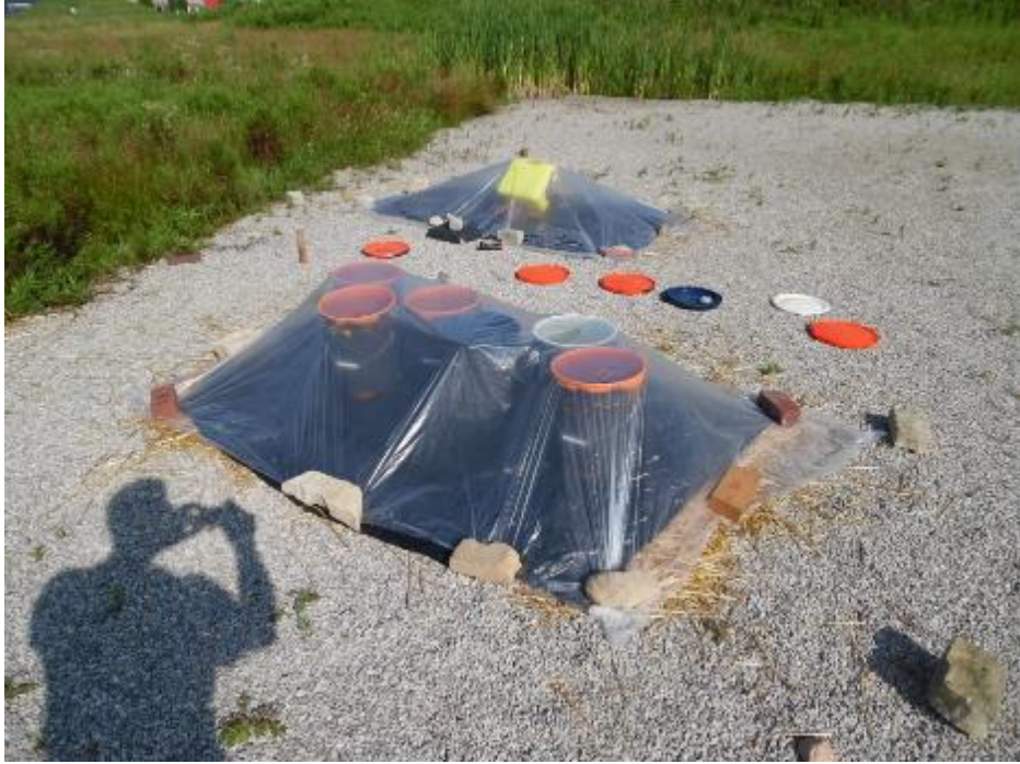
Figure 5: The finished system, on this day heating 6 full buckets of water. The edges of the top layer are held down by rocks, bricks, or logs, with a total of about 12 objects being used.
