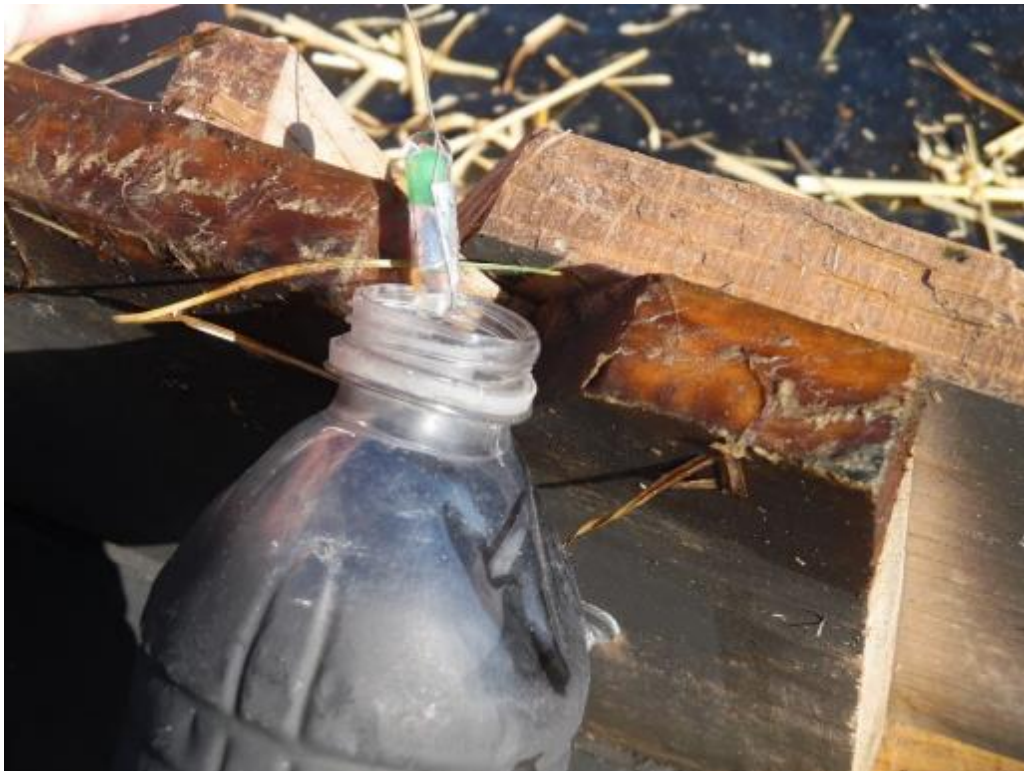
Figure 12: This shows a WAPI (Water Pasteurization Indicator) about to go into the top of a small water bottle. The green wax is in the high end of the sealed glass tube. If the tube comes out later with the wax in the bottom end of the tube, then the water is pasteurized.
