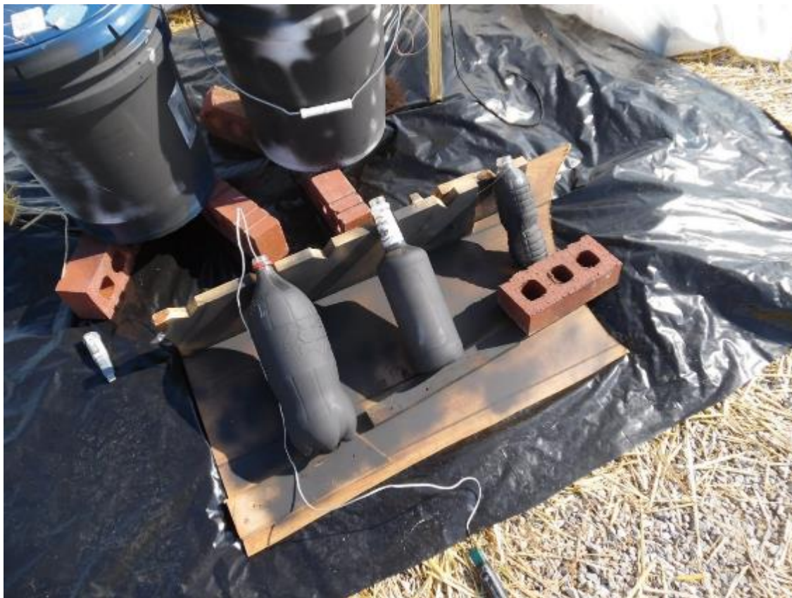
Figure 11: This shows 3 sizes of bottles that can pasteurized. Glass or plastic can be used. The bottles must be angled, as the water at the bottom of the bottle will be significantly cooler than at the top. Painting the bottles black is best, but they work reasonably well in their natural color.
