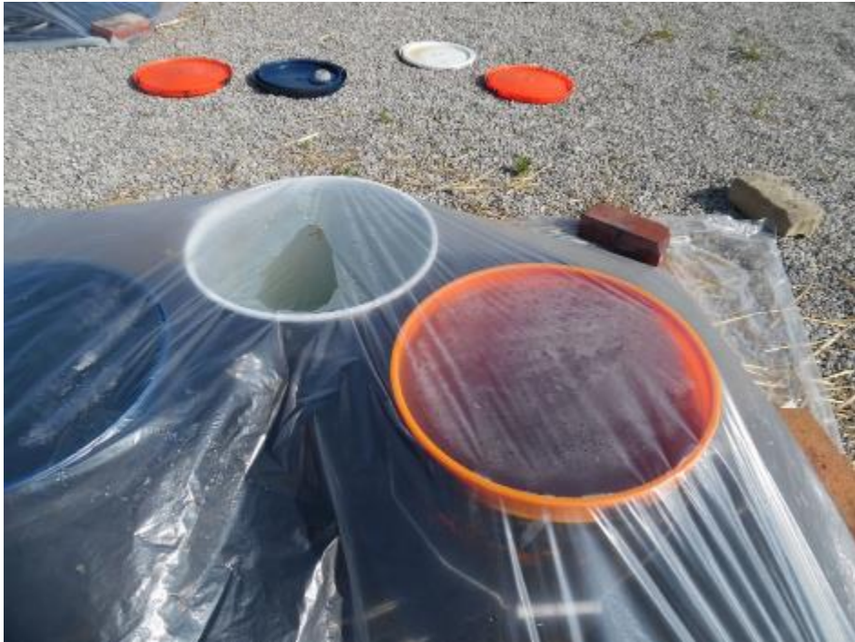
Figure 6: This shows the details of the plastic cover over the top of the open buckets. The plastic should be somewhat snug over the top of the bucket, but it does not need to form a perfect seal. It makes little difference whether the top plastic touches the water or not, the temperature of the white bucket was measured to be essentially the same as the orange and blue buckets.
