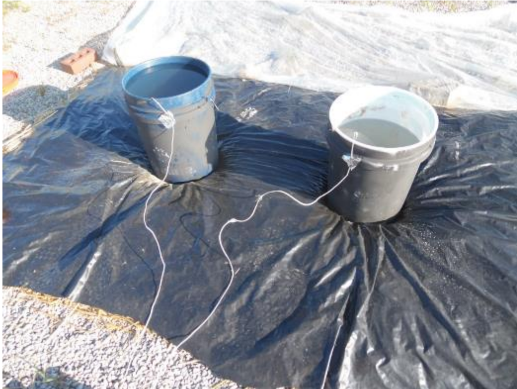
Figure 4: Two buckets to be heated, one full and the other \frac{3}{4} full. The buckets have temperature logging instruments for test purposes.
