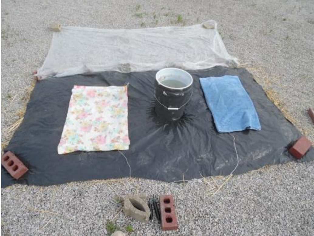
Figure 20: Arrangement for using the heater to kill insect eggs. There is a temperature logger under each stack of clothing.
