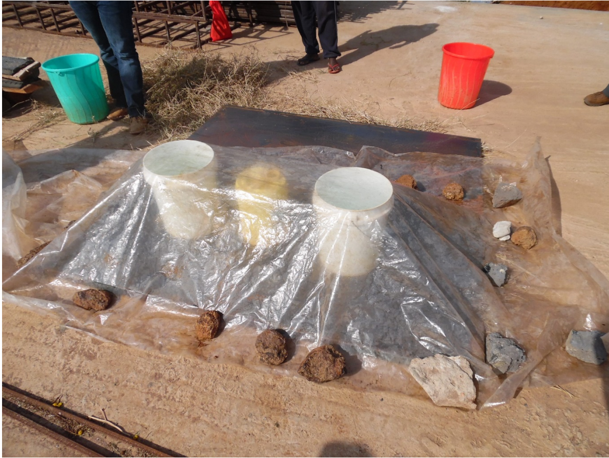
Figure 9: A Solar Household Energy Bank set up in the field using materials that were available. Inside the collector are two large buckets and a 10-liter jerrycan.
