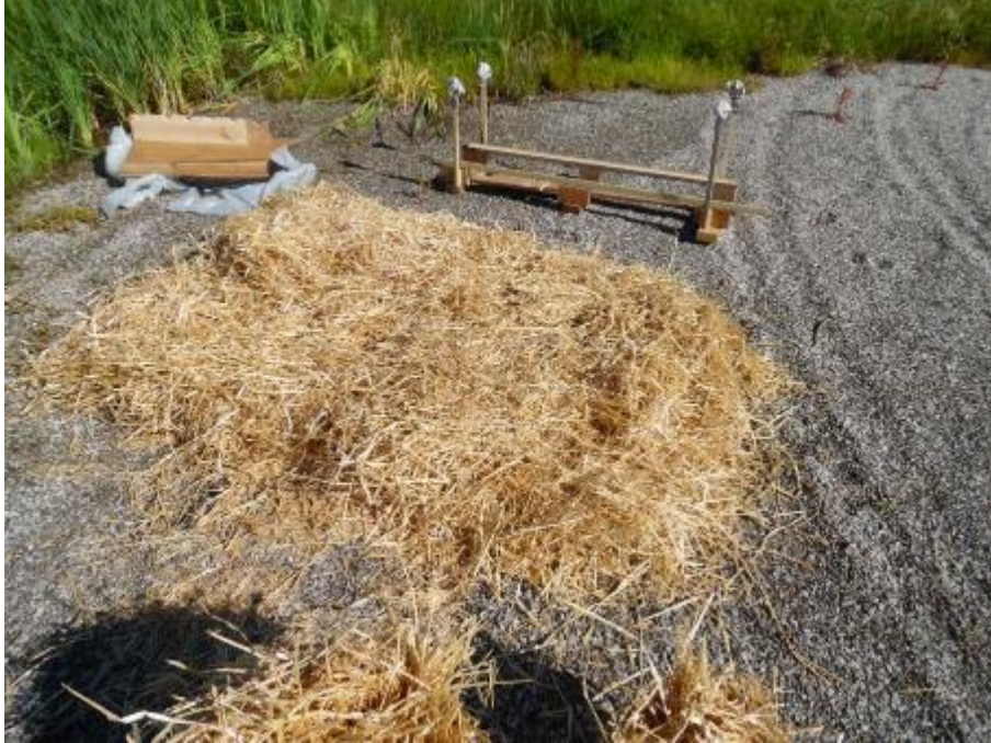
Figure 2: A layer of loose organic material is laid down about 5 cm deep, and about 2.4 m by 1.4 m.
