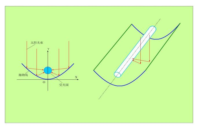
Focus sunlight to the wall of pipe vacuum, the light absorption layer of light energy is converted into heat. High vacuum insulation, so as to achieve above 300 °C high temperature.
