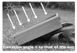
The unit will now heat the water bottles up to 150°F / 66°C and achieve pasteurization in approximately 2 hours. During this heating cycle the unit can be repositioned again to further maximize the solar input. The thermal indicators will reach this temperature when the wax melts and falls to the bottom of each glass tube. Now the colored wax can be seen below the bottom of the bottles, indicating that the water has been successfully disinfected.
