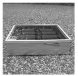
Place the unit so that the orientation (east, south or west) is the same as the sun, and make sure the elevation angle of the unit is equal to that of the sun. This will maximize the amount of solar rays entering the unit and speed the heating process.
