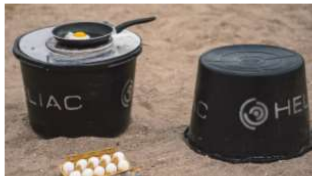
Figure 4: SunStore Cooker with an insulation
