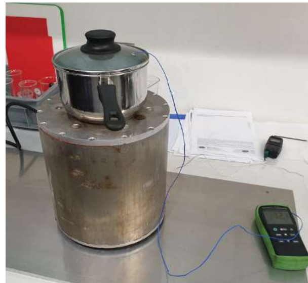
Figure 2: SunStore Cooker tested in the laboratory without insulation
