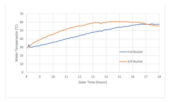
This shows temperature logger traces for two buckets of water on a sunny day, one full and one ¾ full. Nearly the same temperature was achieved, though the less full bucket achieved this temperature first.
