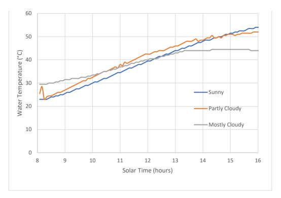
This graph shows bucket temperatures in three types of weather. In all cases, the bucket was 20 liters, full.
