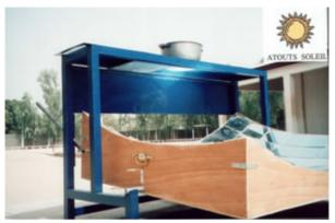
Photo 2: Table underneath view The galvanized shutter is slid to the left of the hole.
