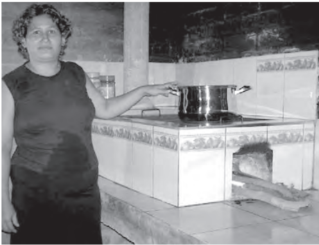
Figure 28: Example of a stove that has been personalized with a ceramic exterior. Photo courtesy of Agua, Arboles y Pueblo, El Salvador
