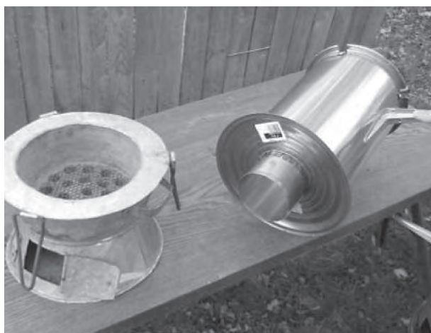
Figure 27: TChar (type of TLUD).
