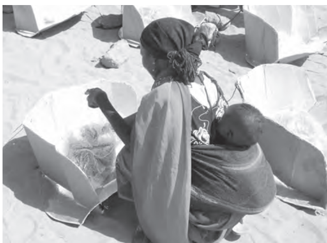
Figure 5: Panel solar cooker. Photo courtesy of Solar Cookers International
