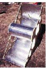
Solar Grill is another new entry to this site. The source is from http://www.tammock.ch/en/index.html . Details are not available, but photo indicates that the device works. The device has a large cylindrical parabolic reflector, with a central chamber for the housing items to be grilled.
