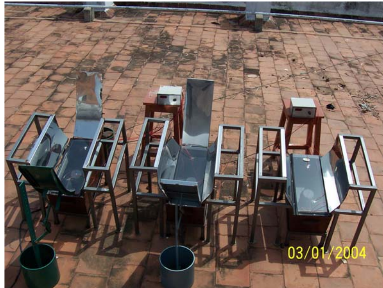
Fig. 7 Schematic diagrams of Solar CPCs with parabolic, linear End-Wall reflectors and without End-Wall reflectors
