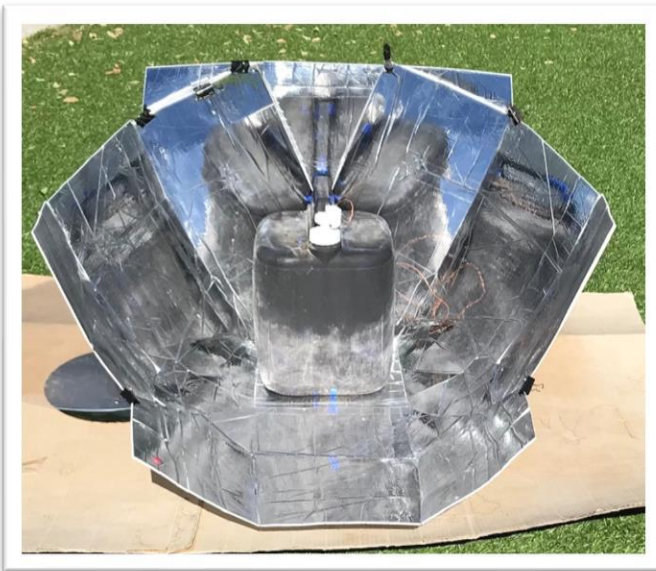
The Haines “triple angle” prototype pasteurizing a 5-gallon jerrycan of water. Photo credit: Roger Haines
