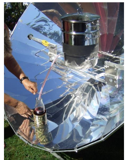
Photo E8: Steam juicer heated by the solar cooker
