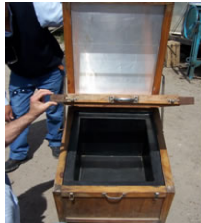
Fig. 7 Cooker with reflective lid
