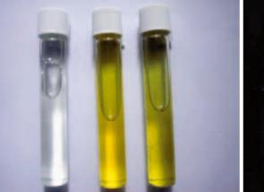
**Figure 4:** Colilert tubes after incubation. The clear tube on the left has no coliforms; the two tubes on the right have some type of coliform bacteria. Photo © Robert H. Metcalf
