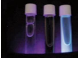
**Figure 5:** The three Colilert tubes after incubation with a UV light shining on them. The center tube does not fluoresce and thus has only environmental coliforms. The tube on the right fluoresces, indicating the presence of E. coli. Photo © Robert H. Metcalf
