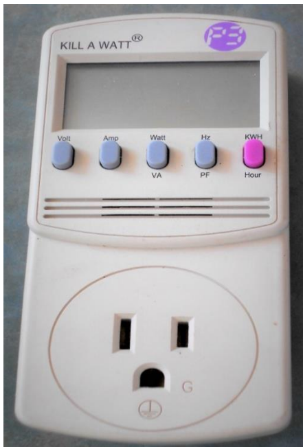
Photo 6. One of the commercial Energy Meter, KILL A WATT (a) Oven and connection to oven (b) for measuring electric energy used.
