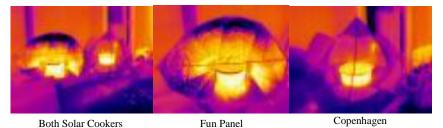
Figure 1. Thermal image of Fun Panel on left and Copenhagen Solar Cooker on right.
