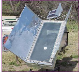
With such a fortunate set of circumstance the reflectors can be folded to cover the cooking chamber making the cooker portable! Mirrors have a reflection of about 99% but lose 5% each time the light passes through the glass. Polished metal surfaces have about 90% reflection but no losses due to glass. The result is that each behaves about the same.
