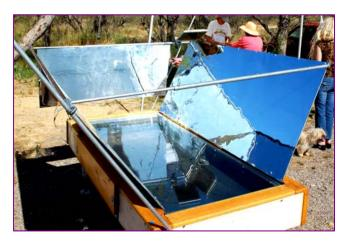
reflective. The penetration into the cover glass improves somewhat because of the more vertical angle. Of the five factors affecting a cooker's cooking temperature three of them were thermal losses. Transmitted losses are controlled with insulation.
