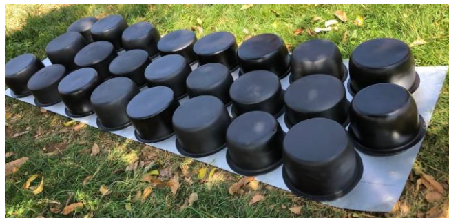
The aluminium pots are sprayed with stovepipe paint on the outside
