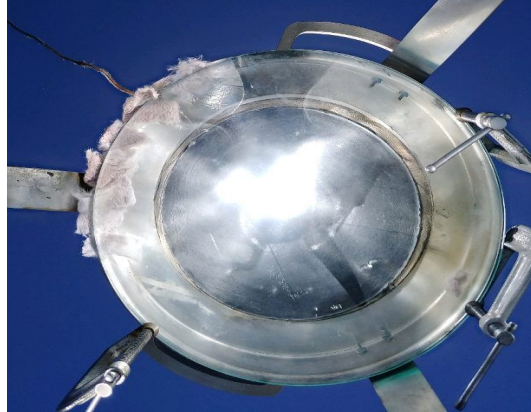
Direct the dish to the sun to concentrate sun rays onto heating plate
