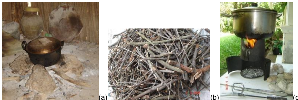
Fig. 8: (a) The 3-stone fireplace; (b) A renewable harvested firewood for cooking with the green stove; (c): The green stove is used to boil 5 litres of water [5]. Portability and self regulating air supply are the advantages.
